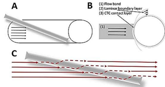
**Figure 2:** (A) Inclined position of the DC01 in the vein. (B) Cross-section of a cylinder that is perpendicular to the incoming flow. (C) Two flow components along inclined DC01.
