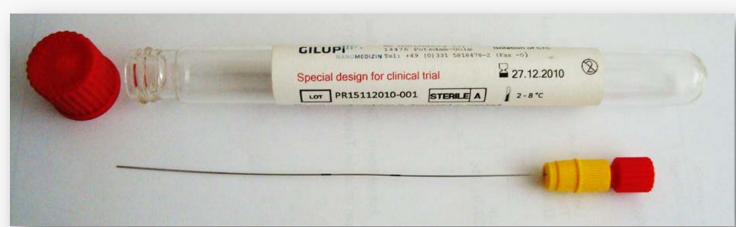
Figure 1: GILUPI Nanodetector for the isolation of rare cells
